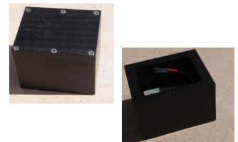
Suitable sensors enclosure for paved roads
