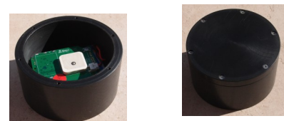
Suitable sensors enclosure for surface asphalt installation
